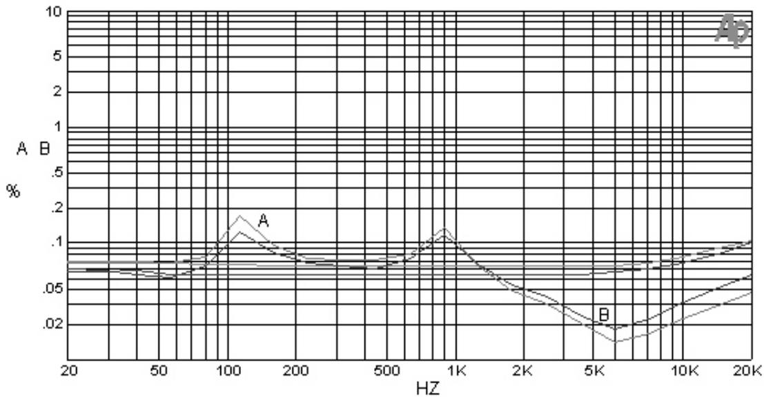
**1 WATT THD VS FREQUENCY WITH 8 OHMS / TOUGH LOAD
