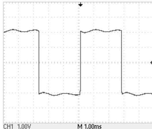
**F7 SQUARE WAVE INTO 1MH + 50 UF SERIES LOAD
