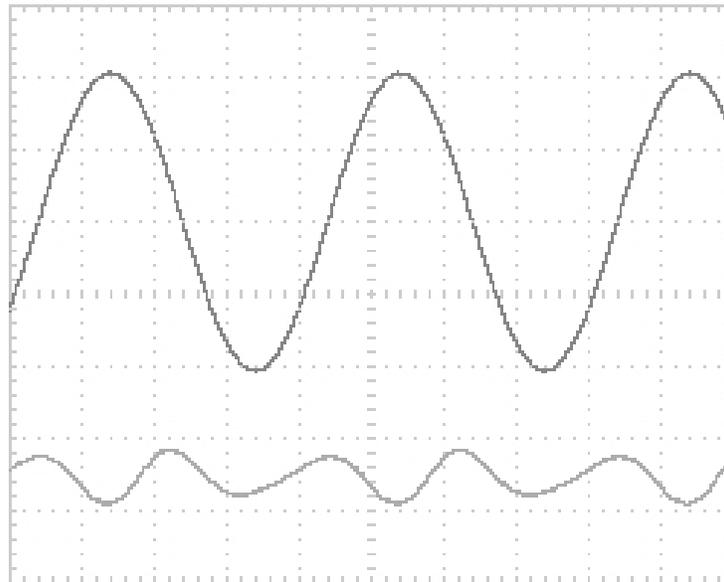
DISTORTION WAVEFORM AT 1 W / 1 KHZ
