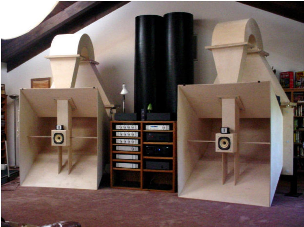
EI Pipe-O is basically two big lengths of 24 inch diameter Sonotube with 21 inch woofers at the bottoms and damped with Dacron or Polyfill. They easily go down to 20 Hz, but their transient characteristic is not so good up around 100 Hz, so you can imagine them as an ideal match. Any room that can hold KleinHorns can find some space for EI Pipe-O, and the over-the-top approach tends to appeal to the same builder.
