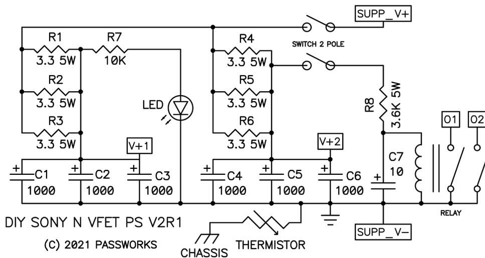
You will note the more elaborate filtering, made necessary by the VFET's exposure to rail noise and the larger thump of the circuit on turn-on/off.
