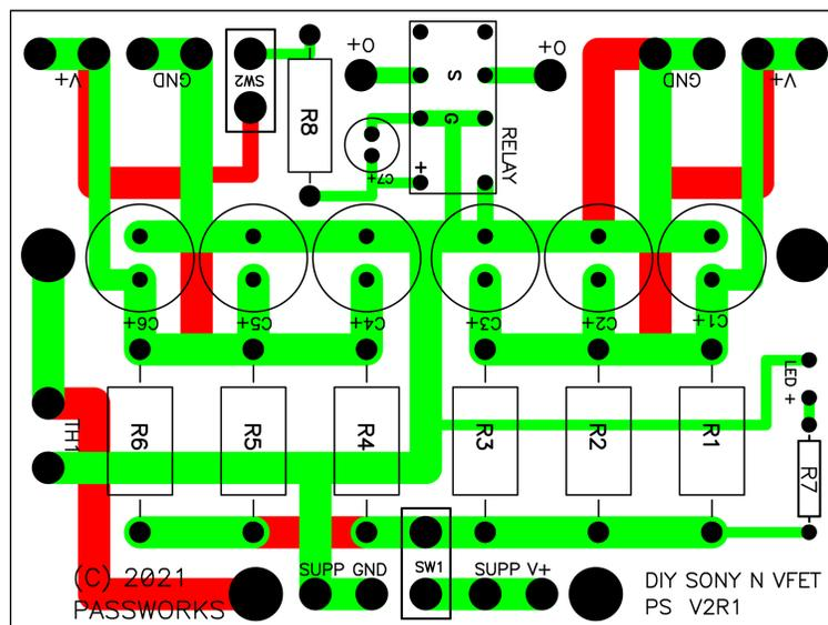
Here is the wiring diagram showing the wiring between components:
