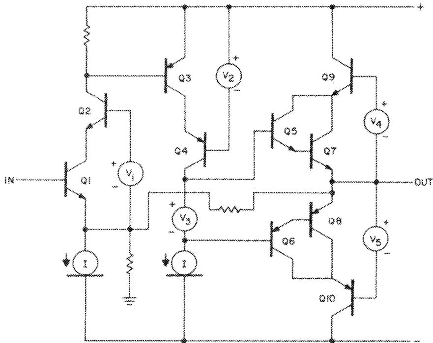
Fig. 9—Basic configuration of the cascode power amplifier.
