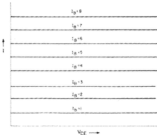
Fig. 2— Actual transistor characteristics.
