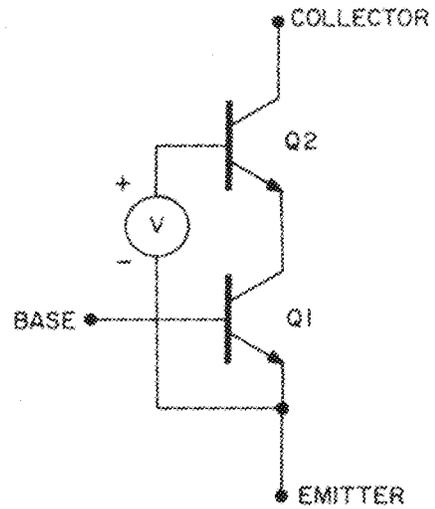
Fig. 4—Cascode operation of transistor Q<sub>1</sub> by the common-base connection of Q<sub>2</sub>.
